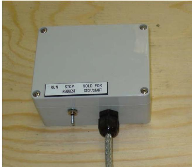
**Figure 2:- Brake Control Switch**
